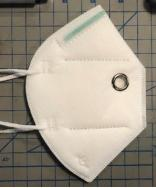
Ensure that the grommet components are pounded tightly together, with the mask fabric secured tightly between the grommet eyelets.
