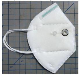
8. Insert the Saliva Ejector nozzle (11/32" outer diameter) into the mask's open grommet hole:
