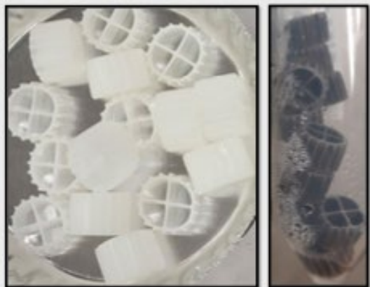
Figure 1. Plastic media (left) are stirred throughout the tanks of the biological treatment system to allow a surface area for bacterial growth. For this project, we collected weekly samples from the tanks and froze them in 50mL Falcon tubes. These media, which are covered with black microbial biofilms (right), are used for both DNA extraction and sequencing, as well as seeding culturing attempts where the only carbon source is 1,4-dioxane.
